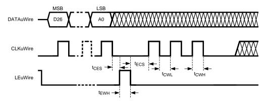
Figure 11. MICROWIRE Timing Diagram: Extra CLKuWire Pulses for R0 to R5
