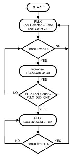
Figure 19. Digital Lock Detect Flowchart
