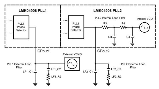
Figure 24. PLL1 and PLL2 Loop Filters
