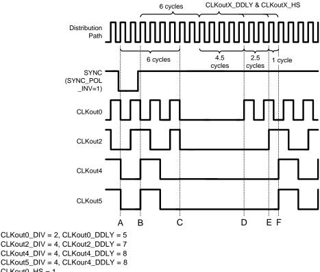
CLKout2\_DIV = 4, CLKout2\_DDLY = CLKout4\_DIV = 4, CLKout4\_DDLY = CLKout5\_DIV = 4, CLKour4\_DDLY = CLKout0\_HS = 1
