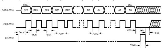
Figure 10. MICROWIRE Timing Diagram
