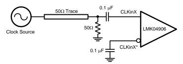
Figure 32. CLKinX/X\* Single-ended Termination
