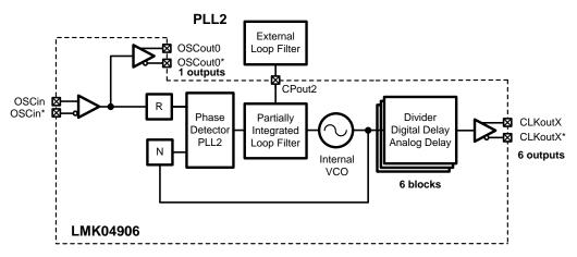
Figure 5. Simplified Functional Block Diagram for Single Loop Mode
