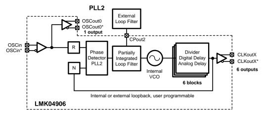
Figure 6. Simplified Functional Block Diagram for 0-delay Single Loop Mode
