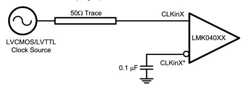
Figure 33. DC Coupled LVCMOS/LVTTL Reference Clock
