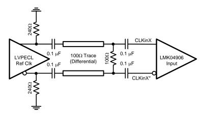
Figure 30. CLKinX/X\* Termination for an LVPECL Reference Clock Source
