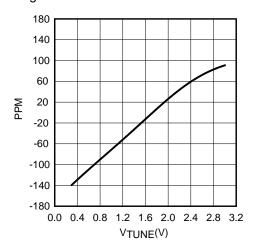
Figure 28. Example Tuning Curve, 20.48 MHz Crystal
