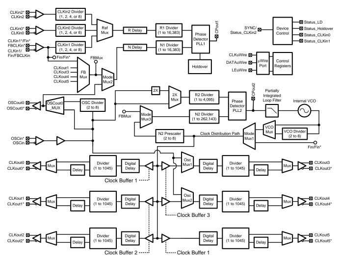
Figure 8. Detailed LMK04906 Block Diagram
