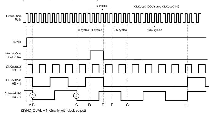
Figure 22. Absolute Dynamic Digital Delay Programming Example
