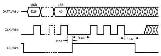
Figure 12. MICROWIRE Timing Diagram: Extra CLKuWire Pulses for R0 to R5 with LEuWire Asserted
