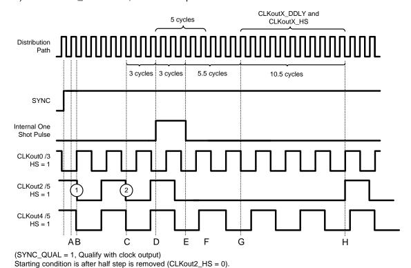
Figure 23. Relative Dynamic Digital Delay Programming Example—2nd adjust
