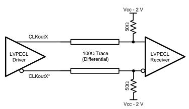
Figure 35. Differential LVPECL Operation, DC Coupling
