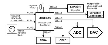
Figure 2. Simplified LMK04906 Block Diagram
