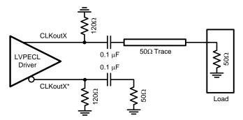
Figure 42. Single-Ended LVPECL Operation, AC Coupling
