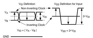
Figure 14. Two Different Definitions for Differential Input Signals
