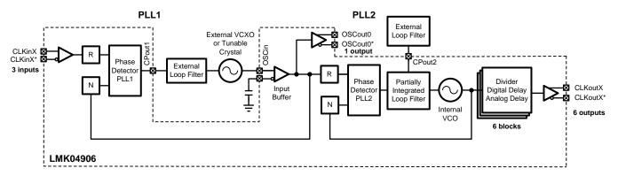
Figure 3. Simplified Functional Block Diagram for Dual Loop Mode
