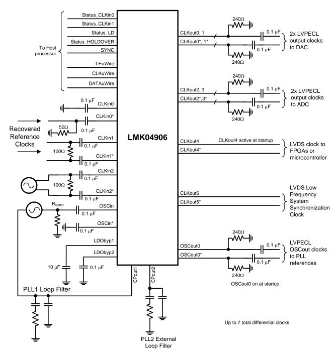
Figure 25. Example Application – System Schematic Except for Power
