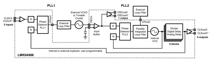
Figure 4. Simplified Functional Block Diagram for 0-delay Dual Loop Mode
