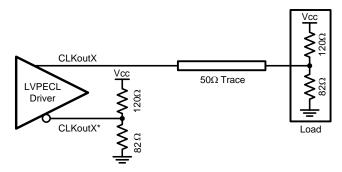
Figure 41. Single-Ended LVPECL Operation, DC Coupling, Thevenin Equivalent
