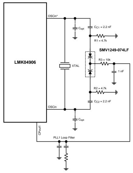
Figure 27. Reference Design Circuit for Crystal Oscillator Option
