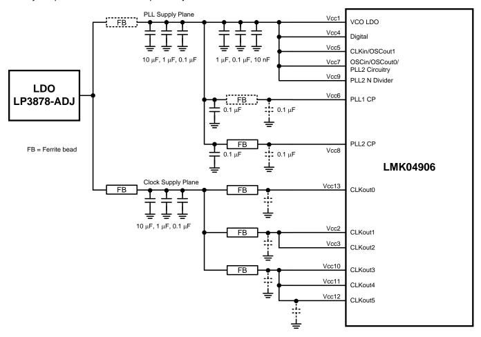
Figure 26. Example Application – Power System Schematic
