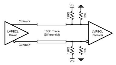
Figure 36. Differential LVPECL Operation, DC Coupling, Thevenin Equivalent
