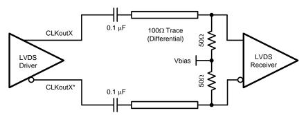
Figure 37. Differential LVDS Operation, AC Coupling, External Biasing at the Receiver
