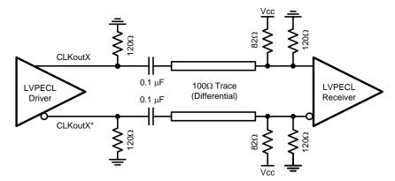
Figure 39. Differential LVPECL Operation, AC Coupling, Thevenin Equivalent, External Biasing at the Receiver
