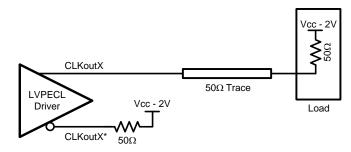
Figure 40. Single-Ended LVPECL Operation, DC Coupling
