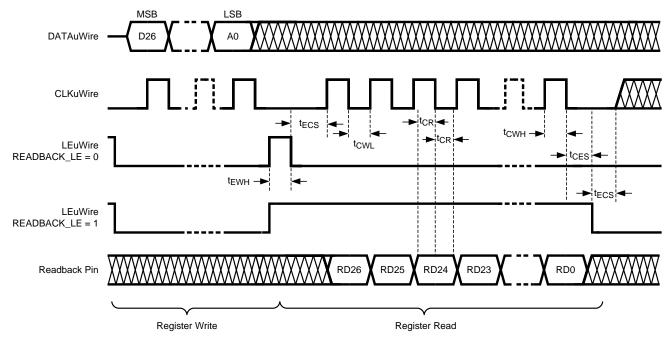
Figure 13. MICROWIRE Readback Timing Diagram
