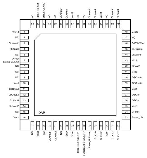
Figure 9. 64-Pin WQFN Package
