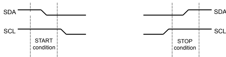
Figure 15-3. START and STOP Conditions
