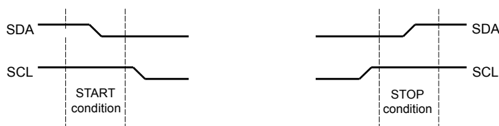
Figure 15-3. START and STOP Conditions
