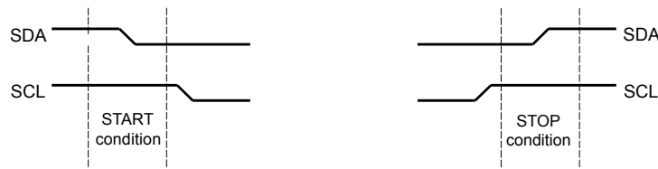
Figure 15-3. START and STOP Conditions
