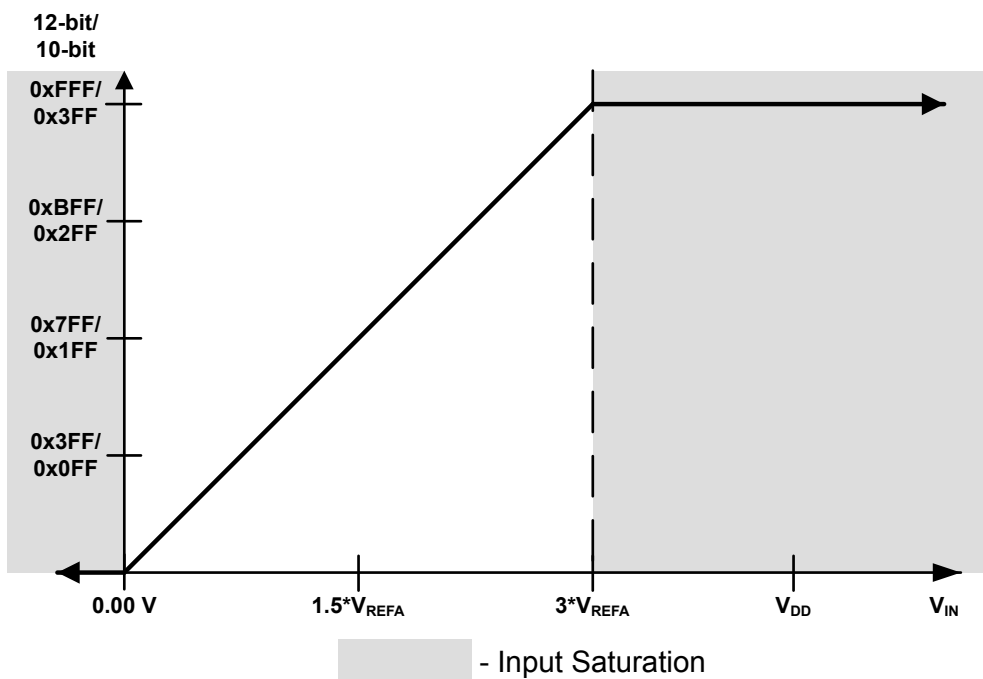
Figure 12-7. External Voltage Conversion Result with 1.0-V Setting
