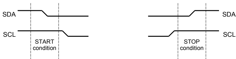
Figure 14-3. START and STOP Conditions
