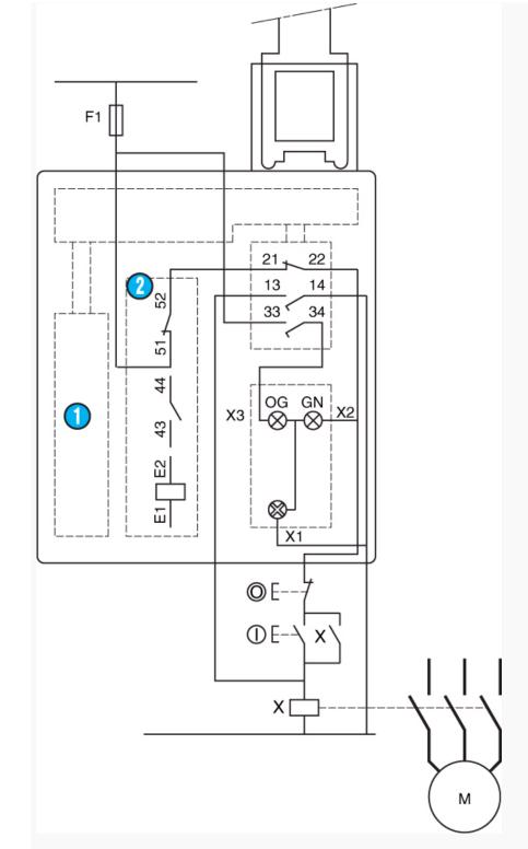
Examples of wiring diagrams with a fuse to provide protection against short-circuits in the cable or tampering. Locking by removal of voltage "NC+NO+NO" 83 894 12
