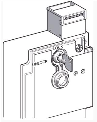
Type 83 894 1 safety switches are supplied with a key-operated lock which can be used to unlock the moving guard, bypassing the electromagnet.
