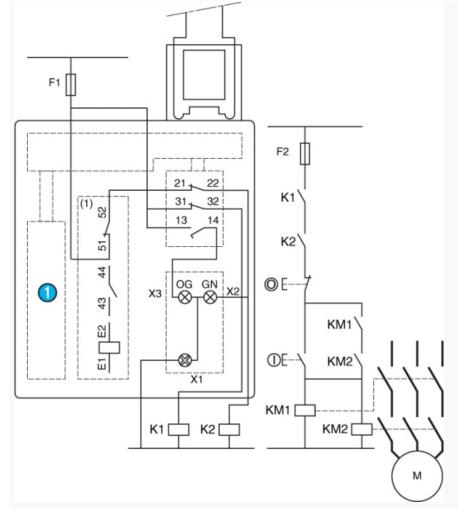
Examples of wiring diagrams with redundancy of the switch contacts, without monitoring. Locking by removal of the voltage "NC+NC+NO" 83 894 13
