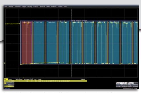
Color-coded overlaid protocol decode makes it easy to understand your serial data messages.
