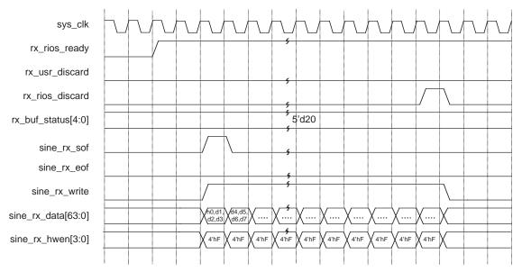
Figure 17. Discarding the Packet using rx\_usr\_discard
