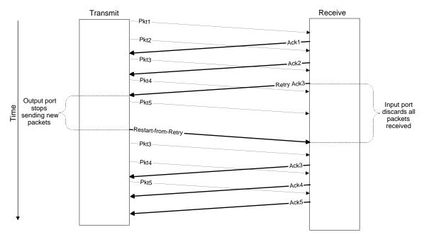
It is possible that by the time the transmitter receives the packet-retry control symbol (RetryAck3), it is still transmitting packet to the receiver due to the transmitter latency to process the packet-retry control symbol. This condition is fine since the receiver discards all incoming packets received after it sends packet-retry control symbols. For more information on the retry recovery state machine, refer to the Serial RapidIO specifications
