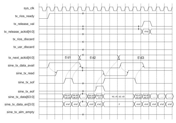
Figure 13. TX Discarding a Packet by tx\_usr\_discard
