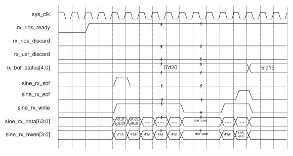
Figure 16. Discarding the Packet using rx\_rios\_discard
