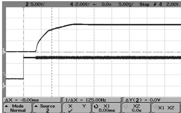
Power On Startup Delay Output ( V_{in} = 0 to 48V, I_{out} = 25A , C_{load} = 0 , T_a = +25^{\circ}C )
