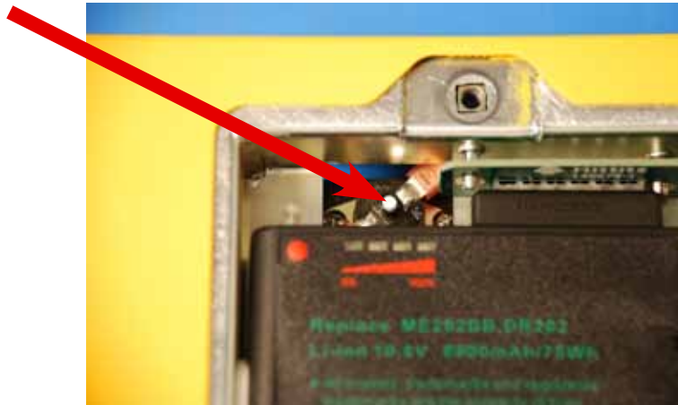
Figure 2. View of thermal switch reset button in T2220B battery compartment
