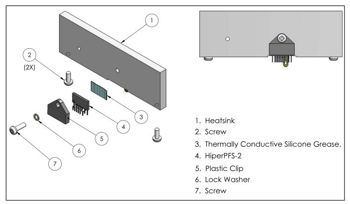
Figure 18. Heat Sink Assembly – With Plastic Clip.
