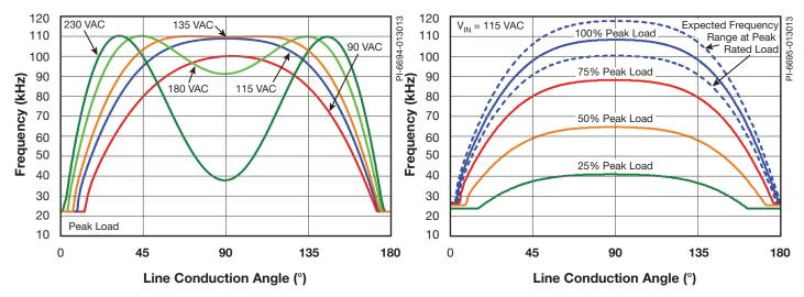
Figure 9. (a) Frequency Variation Over Line Half-Cycle as a Function of Input Voltage (b) Frequency Variation Over Line Half-Cycle as a Function of Load.
