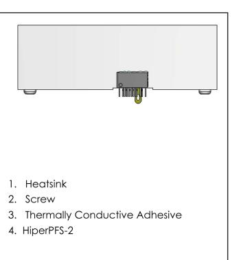
Figure 16. Heat Sink Assembly – Using Thermally Conductive Adhesive.
