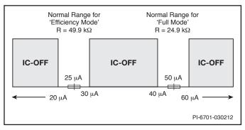
Figure 12. REFERENCE Pin Current Operating Range.
