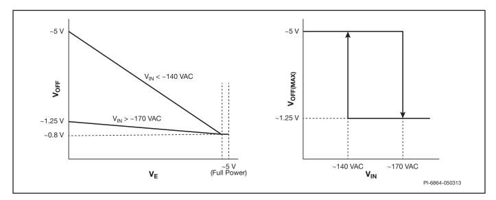
Figure 10. V<sub>OFF</sub> vs. V<sub>E</sub> and V<sub>OFF</sub> vs. Input Voltage.
