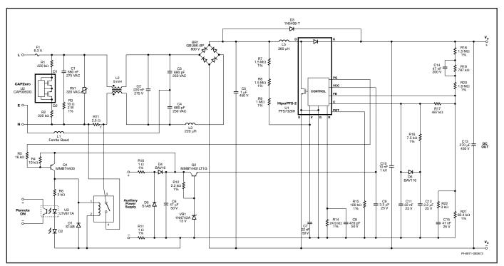
Figure 14. 350 W PFC using PFS7328H.
