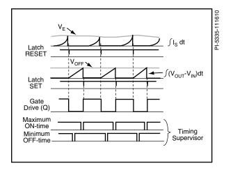
Figure 4. Idealized Converter Waveforms.
