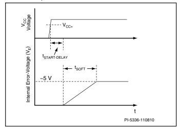
Figure 7. Power Limit Soft-Start Function.
