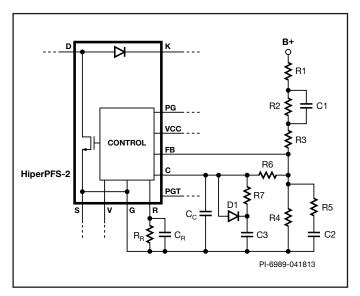
Figure 15. Recommended Feedback Circuit.
