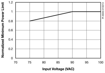
Figure 6. Normalized Minimum Power Limit as Function of Input Voltage.
