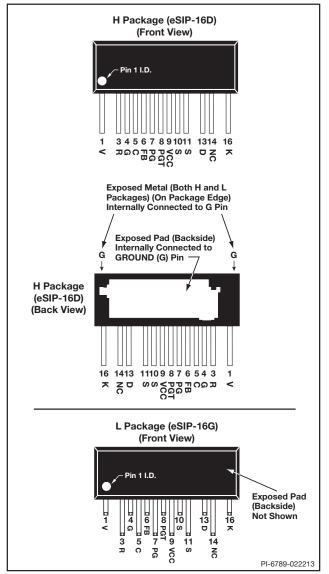
Figure 2. Pin Configuration.
