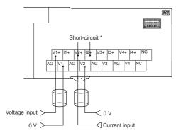
\* Short-circuit the "V positive" terminal and "I positive" terminal at current input.
