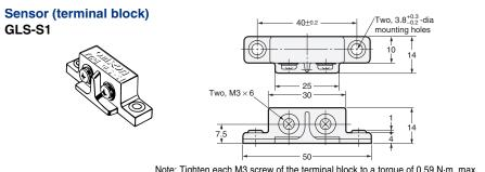
Note: Tighten each M3 screw of the terminal block to a torque of 0.59  $\ensuremath{\text{N}}\xspace{\text{-}}\text{m}$  max.
