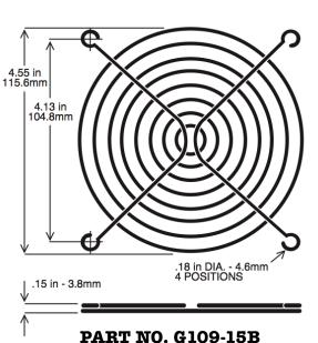
WIRE DIAMETER. RING DIA: 1.8mm RIB DIA: 1.8mm
