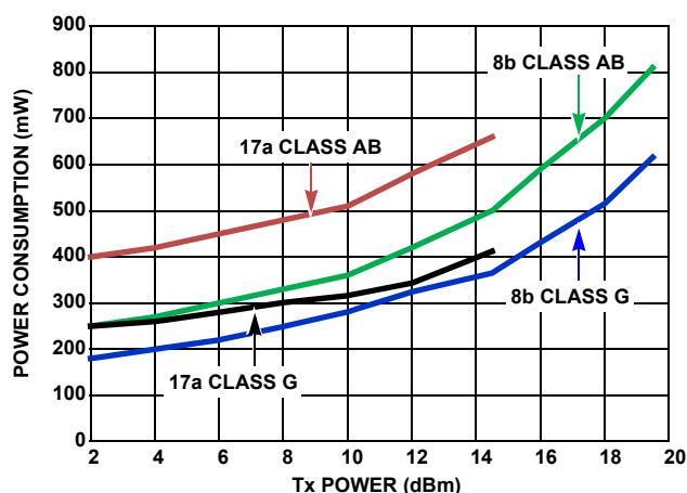
FIGURE 2. CLASS G+ vs CLASS AB DRIVER TOTAL POWER
