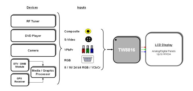
Figure 1 TW8816 Flat Panel TV/Monitor controller system block diagram
