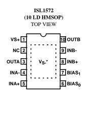
\*THERMAL PAD MUST BE CONNECTED TO NEGATIVE SUPPLY: V<sub>S-</sub>.
