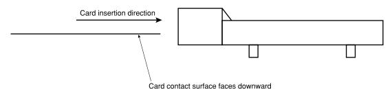
2. After the smart card has been inserted, be sure not to apply excessive force to the card portion that protrudes from the insertion slot.
