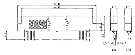
• Recommended board thickness: 0.4 to 0.5mm
