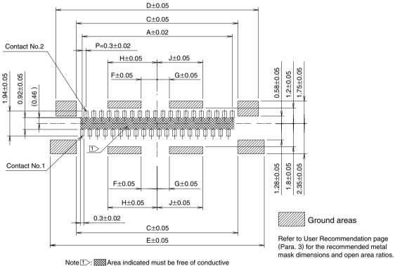
traces or the conductive traces must be covered by resist film.
