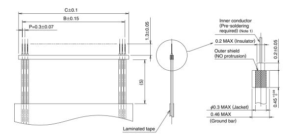
Note 1: Contact Hirose for Termination Procedures.
