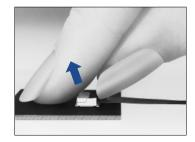
3) Assure that the FPC/FFC is fully inserted parallel to mounting surface, with the exposed conductive traces facing down.
