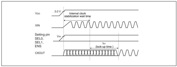
If the setting pin is fixed at the "H" or "L" level, the maximum time after the power is turned on until the set clock signal is output from CKOUT pin is (the stabilization wait time of input clock to XIN pin) + (the lock-up time "tlk"). For the input clock stabilization time, check the characteristics of the resonator or oscillator used.
