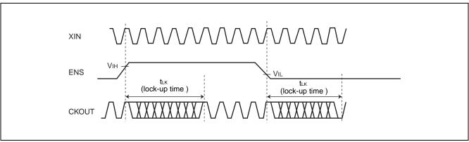
For modulation enable control using the ENS pin during normal operation, the set clock signal is output from CKOUT pin at most the lock-up time (tlk) after the level at the ENS pin is determined.
