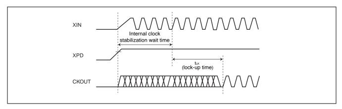
When the power down is controlled by XPD pin, the desired clock is obtained after the pin is set to H level until the maximum lock-up time tlk is elapsed.
