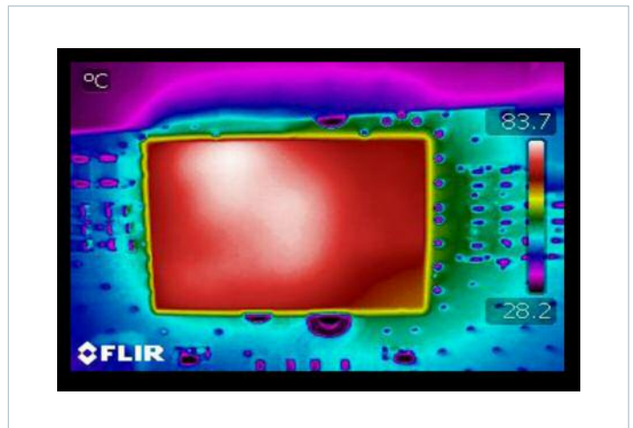
Figure 20 — Thermal Image ( V_{IN} = 28 V, I_{OUT} = 4.2 A, CR, 0 LFM Evaluation PCB)
