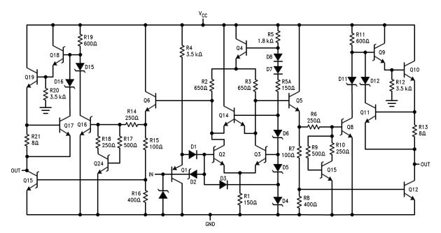
Figure 2. Equivalent Circuit
