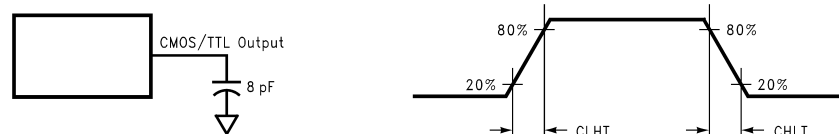
Figure 4. Receiver CMOS/TTL Output Load and Transition Times
