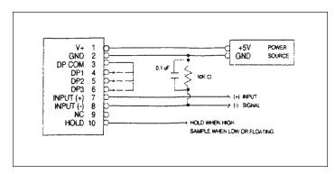
The input common mode range is  $\pm$  1Vdc. If INPUT (–) is not directly conected to GND, a 10k resistor network can be connected as shown to reduce unstable readings.
