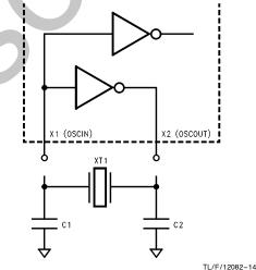
FIGURE 19. Crystal Connection to DP83907 (see text for component values)
