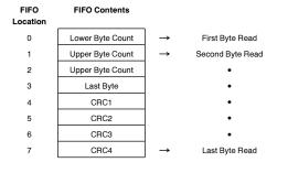
For the following alignment in the FIFO the packet length should be  $(N \times 8) + 5$  Bytes. Note that if the CRC bit in the TCR is set, CRC will not be appended by the transmitter. If the CRC is appended by the transmitter, the 1st four bytes, bytes N-3 to N, correspond to the CRC.
