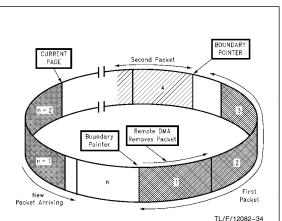
FIGURE 39. 1st Received Packet Removed by Remote DMA
