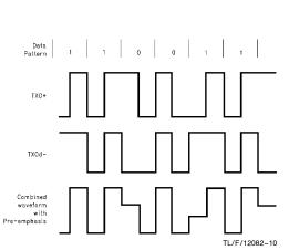
FIGURE 15. Typical Summed Transmit Waveform
