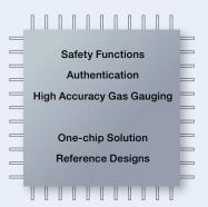
dedicated to Li-lon battery management supporting from 1 to 4 cells in series. This product family offers a unique set of features to optimize performance and security. This includes an outstanding voltage measurement accuracy of ±12.5 mV in the 0 to +60°C temperature range, helping customers to extend the battery energy that can be safely used between
