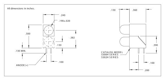
Note: 5390 Series piggy-back block slides onto 5300H block, must be pre-assembled before inserting in PC board.
