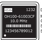
Date Code (YYWW) Model Number **Output Frequency** Serial # Barcode Serial Number
