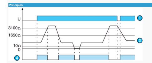
The relay is reset either using the RESET pushbutton on the front face or by opening the external contact S2 (remote reset), or by cutting the auxiliary power supply (terminals A1 - A2). If the auxiliary power is cut for a period of time greater than the reset time (500 ms), the relay is reactivated if the proble detects a normal temperature when the power supply voltage is restored.
