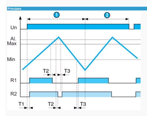
On power-up, the level in the tank is low, relays R1 and R2 are energised and the pump is ON : filling starts, the LED for relay R1 is lit. When the level reaches the Max probe, relay R1 de-energises and the pump is OFF : filling stops, the relay LED goes off. If, in the event of a fault, the level continues to rise and reaches proble AI., relay R2 de-energises and the alarme is triggered : the LED for relay R2 is lit. This fault can be stored.
