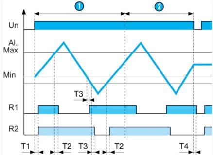
On power-up, probe AI. is submerged, relays R1 and R2 are energised and the pump is ON: filling starts, the LED for relay R1 is lit. When the level reaches the Max probe, relay R1 de-energises and the pump is OFF : filling stores, the LED for relay R1 goes off. Relay R1 re-energises when the Min probe emerges. In the event of a fault (level continues to fall) probe AI. emerges, relay R2 deenergises and the alarme is triggered : the LED for relay R2 is lit. This fault can be stored
