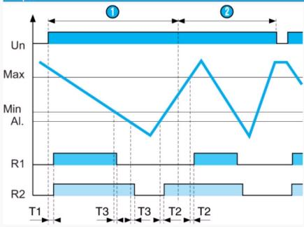
On power-up, probes Min, Max and AI. are submerged, relays R1 and R2 are energised and the pump is ON : emptying starts, the LED for relay R1 is lit. When the Min probe emerges, relay R1 goes off. If, in the event of a fault, the level continues to fall and probe AI. emerges, relay R2 de-energises and the alarm is triggered : the LED relay R2 is lit. This fault can be stored.
