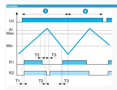
On power-up, the level in the tank is low, relays R1 and R2 are energised and the pump is ON: filling starts, the LED for relay R1 is lit. When the level reaches the Max probe, relay R1 de-energises and the pump is OFF: filling stops, the relay LED goes off. If, in the event of a fault, the level continues to rise and reaches proble AI., relay R2 de-energises and the alarme is triggered: the LED for relay R2 is lit.
