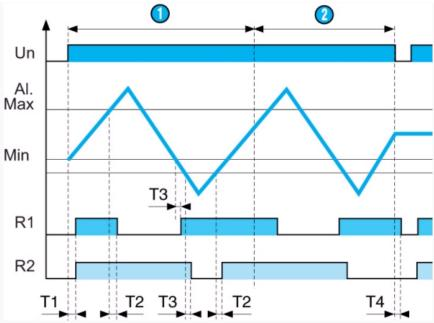
On power-up, probe Al. is submerged, relays R1 and R2 are energised and the pump is ON: filling starts, the LED for relay R1 is lit. When the level reaches the Max probe, relay R1 de-energises and the pump is OFF: filling stops, the LED for relay R1 goes off. Relay R1 re-energises when the Min probe emerges. In the event of a fault (level continues to fall) probe Al. emerges, relay R2 deenergises and the alarme is triggered: the LED for relay R2 is lit.
