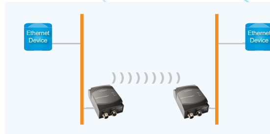
Ethernet Port Adapters (EPA) replacing the ethernet cable with wireless connection. The connection between the EPAs is point-to-point in Bluetooth technology and ad-hoc in Wireless LAN.
