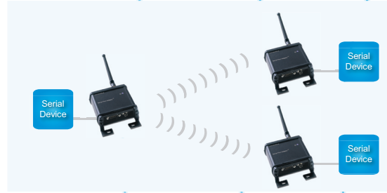
Serial Port Adapters (SPA) replacing the serial cables with wireless connections in point-to-point and multidrop setups.
