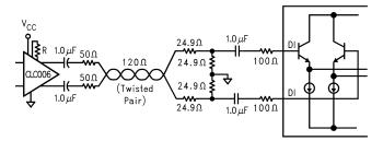
Figure 29. Twisted Pair Equalization
