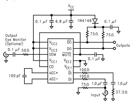
Figure 17. CLC014 Equalizer Application Circuit
