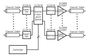
Figure 28. Video Routing Block Diagram
