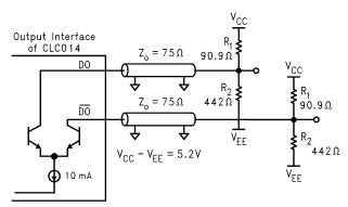
Figure 23. Alternative Load Terminated Output Interface
