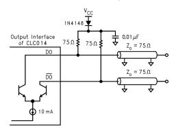
Figure 22. Differential Source Terminated Output Interface
