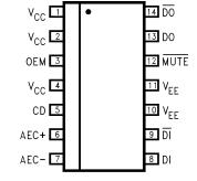
Figure 1. 14-Pin SOIC (Top View) See D Package
