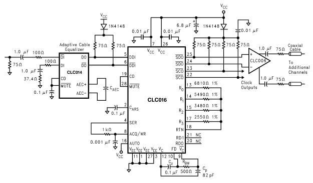
Figure 27. Typical Repeater Design
