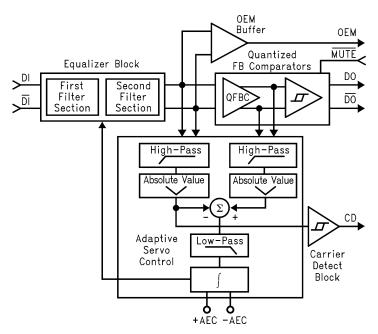
Figure 18. CLC014 Block Diagram
