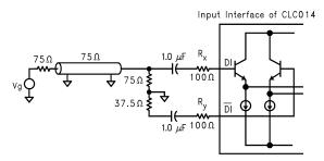
Figure 19. Single-Ended 75Ω Cable Input Interface
