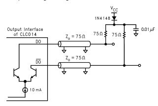
Figure 21. Differential Load Terminated Output Interface
