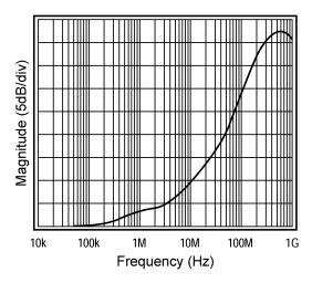
Figure 26. Maximum Equalization Response
