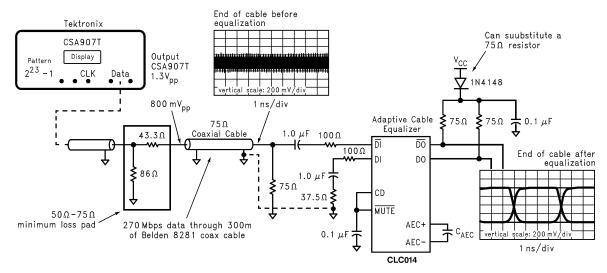
Figure 31. Typical Measurement Setup
