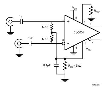
FIGURE 7. Twisted Pair Cable, AC-coupled
