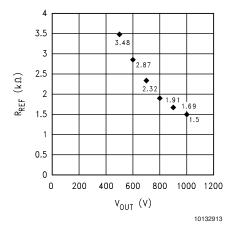
FIGURE 10. Output level's sensitivity to R<sub>REF</sub>
