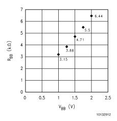
FIGURE 4.  $R_{BB}$  vs.  $V_{BB}$  for  $R_{REF}$  = 1.5  $k\Omega$
