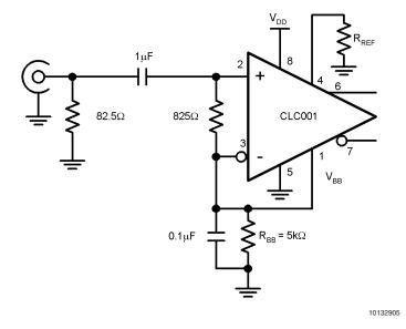
FIGURE 5. Single Ended 75 $\Omega$  Coaxial Cable, AC-coupled
