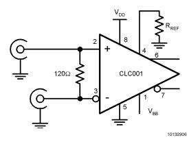
FIGURE 6. Twisted Pair Cable, DC-coupled
