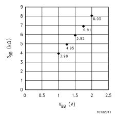
FIGURE 3.  $R_{BB}$  vs.  $V_{BB}$  for  $R_{REF}$  = 1.91  $k\Omega$
