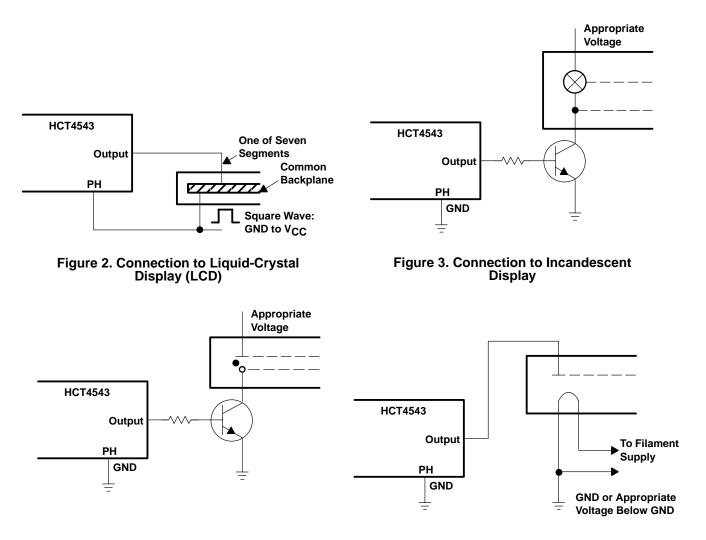
Figure 4. Connection to Gas-Discharge Display
