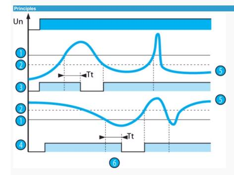
The under or overvoltage threshold value is set by a graduated potentiometer by reading the Un scale to be monitored directly. The hysteresis is set by a graduated potentiometer from 5 to 20 % of the preset threshold. The hysteresis value cannot be higher than the extremes of the measurement range.
