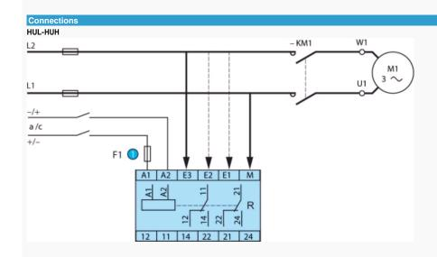
NB : When controlling DC voltage from the same source supplying terminals A1 and A2, terminal M must be connected directly to the "minus" pole of this power supply.
