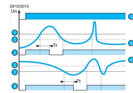
In overvoltage mode, if the controlled voltage exceeds the preset threshold for longer than the time set on the front face (0.1 to 3 s), the output relay opens and LED R is extinguished. During the time delay, this LED flashes.
