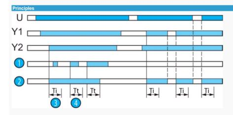
This mode is for controlling a pump based on two external signals (Y1 and Y2). The output relay closes when both input signals are present (Y1 and Y2 closed). It will open as soon as either of these two signals is absent.
