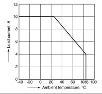
2. Load current vs. ambient temperature characteristics in adjacent mounting I∟: Load current;
