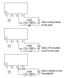
2) Even if spike voltages generated at the load are limited with a clamp diode if the circuit wires are long, spike voltages will occur by inductance. Keep wires as short as possible to minimize inductance.
