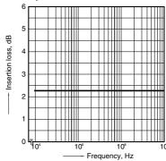
14. Insertion loss vs. frequency characteristics
