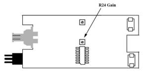
Figure 2, Gain Adjustment Location
