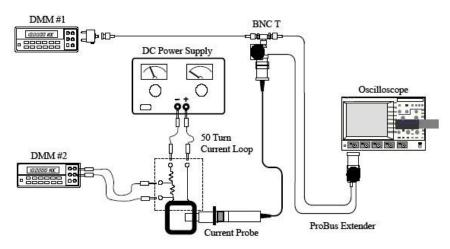
Figure 1, DC Accuracy Test Set Up
