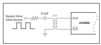
FIGURE 11. Connecting a Ground Referenced Square Wave Clock Source to the ADS808 Using a RF Transformer.
