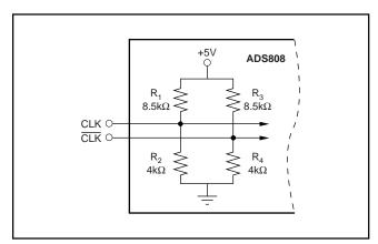
FIGURE 9. The Differential Clock Inputs are Internally Biased.
