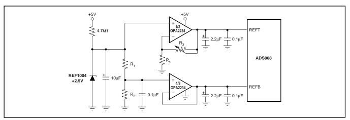
FIGURE 8. Example for an External Reference Circuit Using a Dual, Single-Supply Op Amp.
