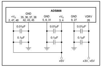
FIGURE 13. Recommended Supply Decoupling Scheme.
