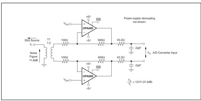
FIGURE 6. Wideband Differential A/D Converter Driver.
