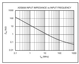
FIGURE 2. Differential Input Impedance versus Input Frequency.
