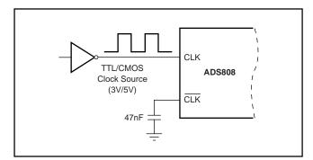
FIGURE 10. Single-Ended TTL/CMOS Clock Source.
