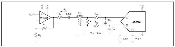
FIGURE 5. Converting a Single-Ended Input Signal into a Differential Signal Using a RF Transformer.
