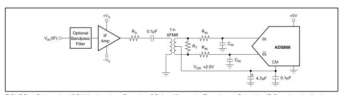
FIGURE 4. Driving the ADS808 with a Low Distortion RF Amplifier and a Transformer Suited for IF Sampling Applications.
