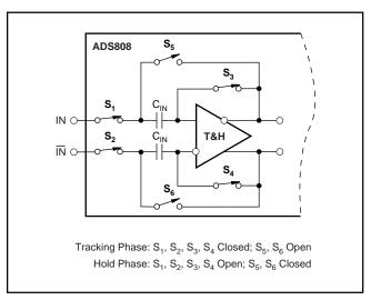
FIGURE 1. Simplified Circuit of Input Track-and-Hold Amplifier.
