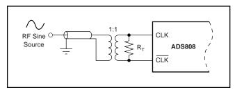
FIGURE 12. Applying a Sinusoidal Clock to the ADS808.
