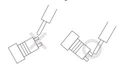
• Leave a gap of at least 1 mm between the soldered parts and the surface of the case so that flux does not get inside the Switch.
