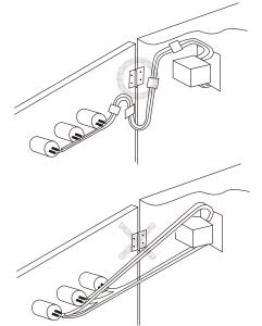
• With miniature Switches, the gap between the terminals is very narrow. Use protective or heat-absorbing tubes to prevent burning of the wire sheath or shorting.
