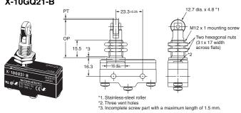
Note: Do not use both the M12 mounting screw and the mounting holes in the case at the same time. Doing so will cause stress to be applied to the Switch, possibly damaging the case or cover.
