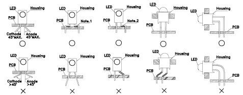
" $\bigcirc$ " Correct mounting method "imes" Incorrect mounting method
