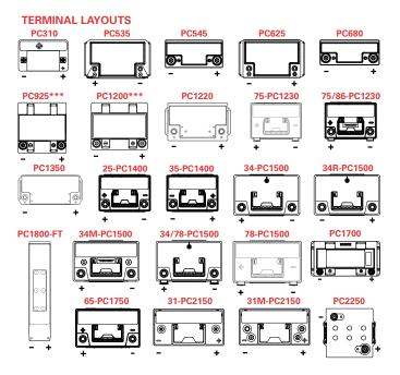
Drawing sizes are for terminal position reference only; diagrams are not proportionate to each other. \*\*\*Optional Reversed Polarity (L)
